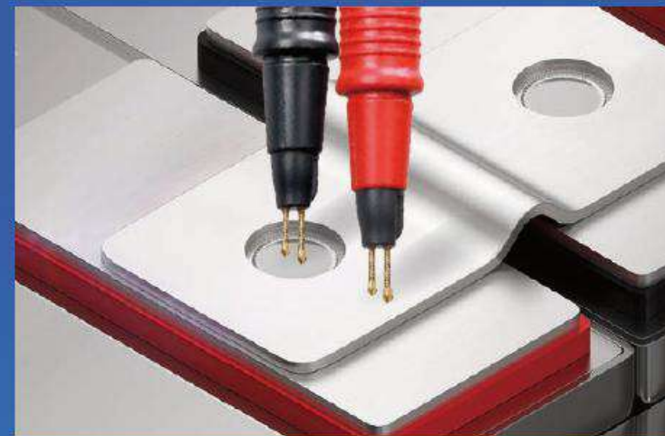
Judges connection quality by measuring resistance
