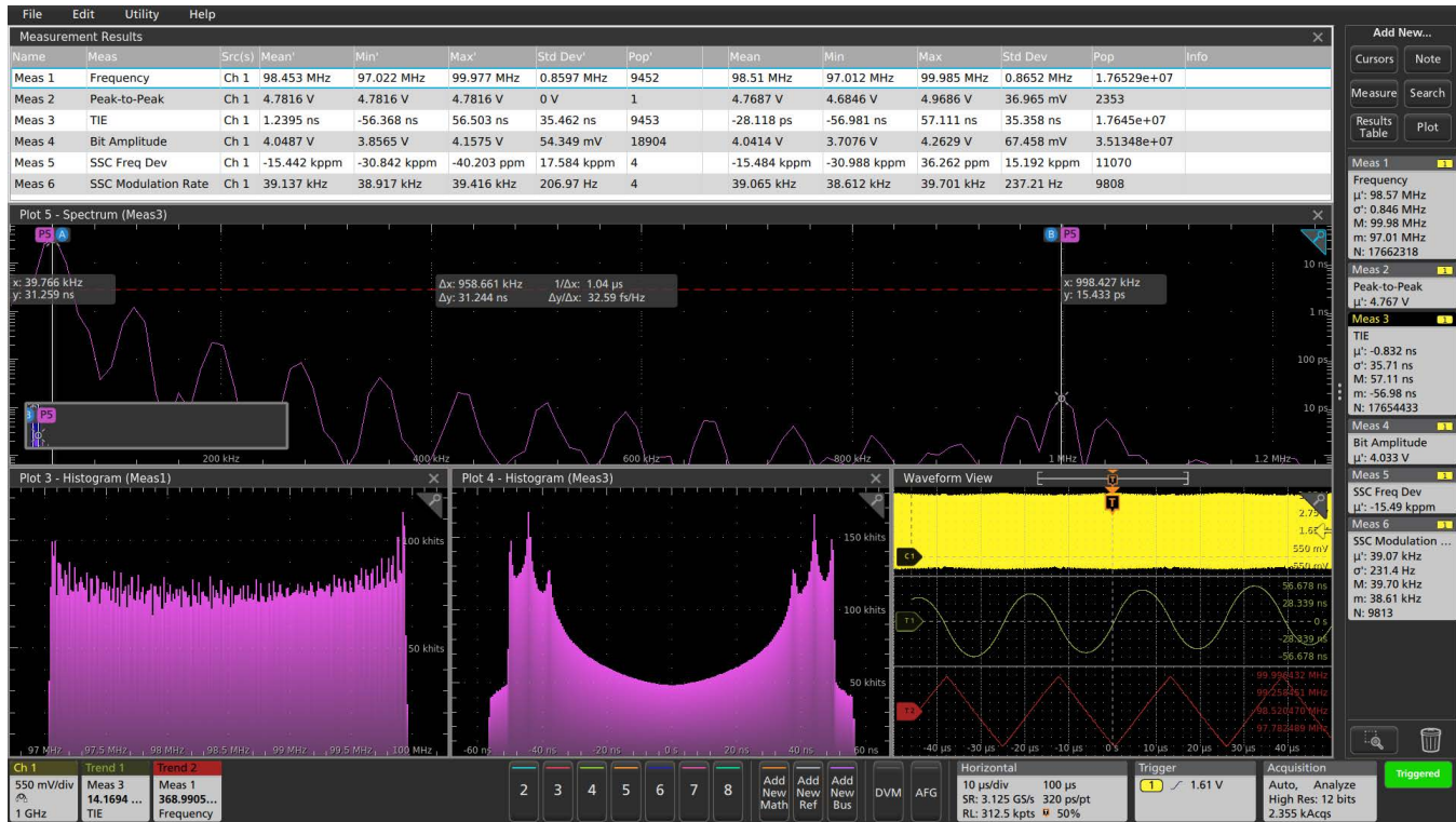
Analysis of a spread spectrum clock signal, showing the 39 kHz triangular modulation on the 98 MHz clock.
