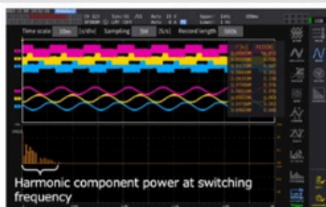
FFT analysis of effective power (up to 6 MHz)
